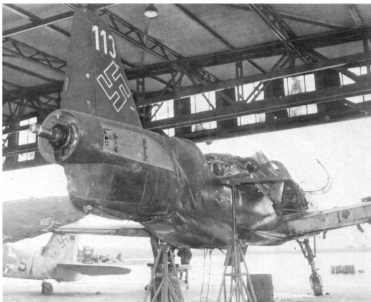
Above: The badly damaged Do 335 A-1 (W Nr. 240113) after it crashed with the night fighter ace, Major Wolfgang Schnauffer at the controls. The airplane, which was undergoing repairs, was captured by US troops at Bindlach near Bayreuth. Below: This Do 335 A-1, photographed in France, is thought to be the second Pfaff brought to the United States aboard HMS Reaper. Interestingly, the aircraft is juxtaposed to the remains of four German jets including three He 162s and an Me 262.
