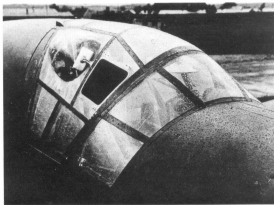
Above: The canopy of the Do 335 pictured after a rain shower. To improve visibility to the rear, a special "teardrop" was fitted to both sides to accommodate a rearview mirror. Forward of this was positioned a square glazed panel which could be opened to further improve visibility. Below: The Do 335 was only the second piston-engined aircraft to be fitted with an ejector seat, compressed air being used to propel the pilot clear of the cockpit in an emergency.
