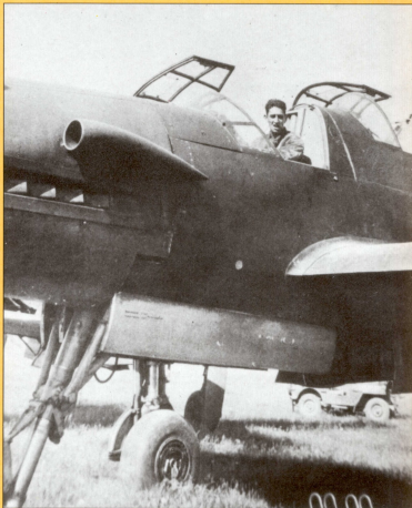
Right: An American soldier seated in the pupil's cockpit of a two-seat trainer, Do 335 A-10 (W. Nr. 240112) after it was transferred to Neubiberg in September 1945. Notice the leading edge near the root of the wing with its sharp edge designed to break the airflow. This was to create better low speed characteristics during the landing cycle.
